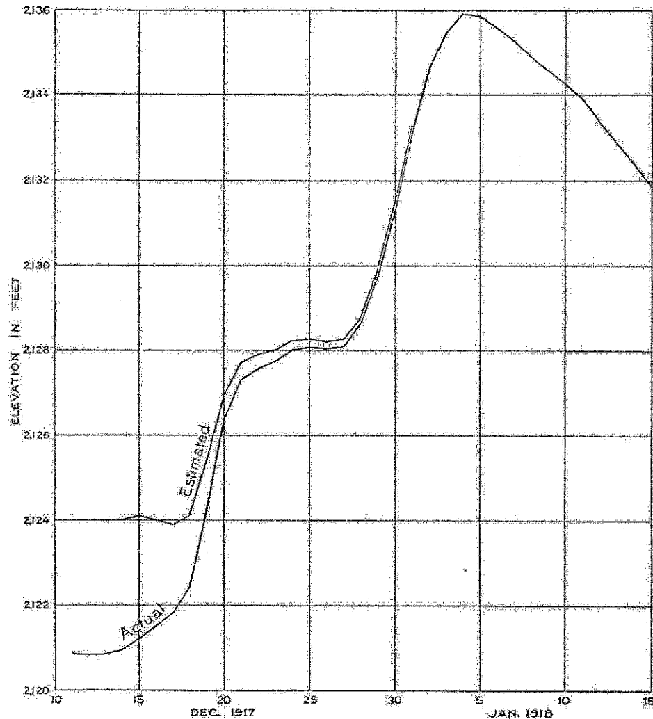
FIGURE 2.—Comparison of actual hydrograph for heights of Coeur d'Alene Lake in flood of January, 1918, and estimated hydrograph assuming storage in lake to level of 2,124 feet at beginning of flood.
