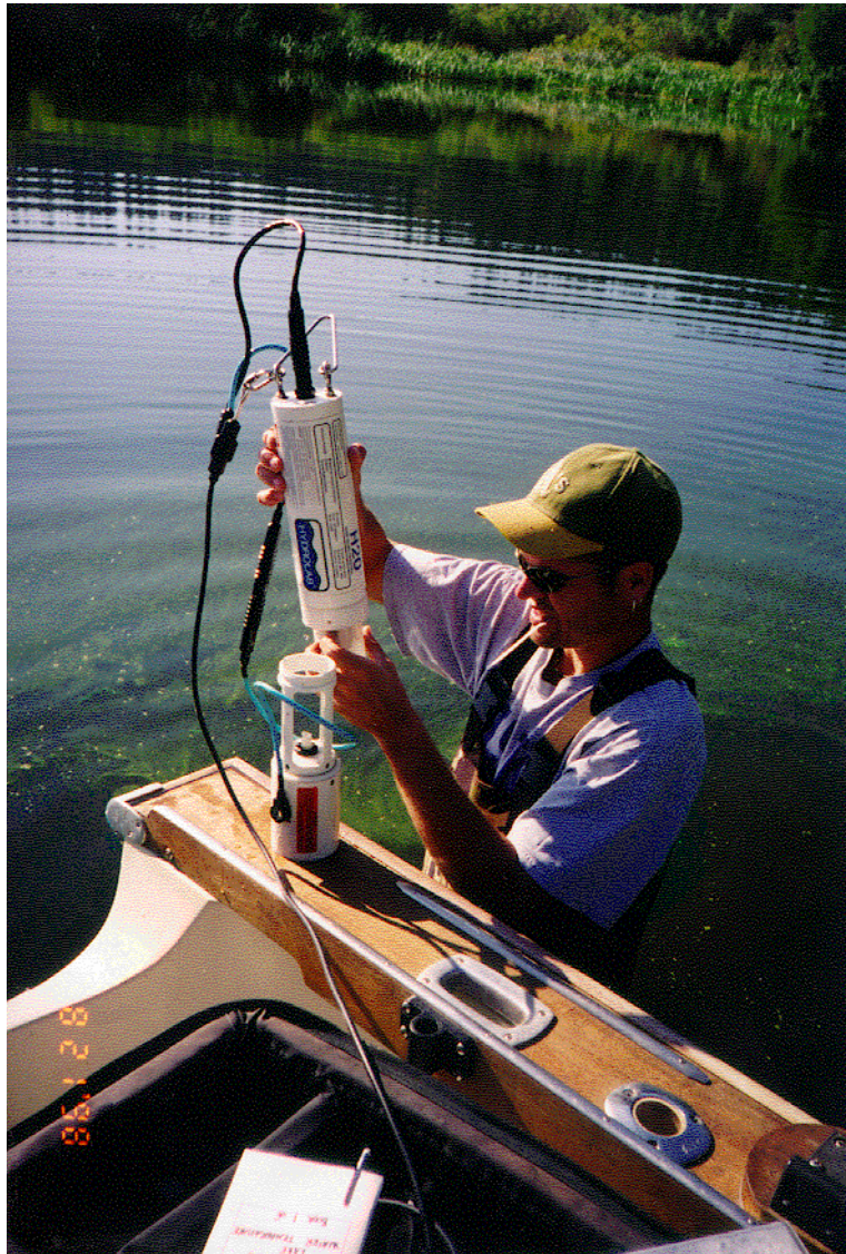
Figure B2. Photo showing measurement of water quality parameters (dissolved oxygen, pH, conductivity, and temperature) in Upper Klamath Lake, August 21, 1998.
