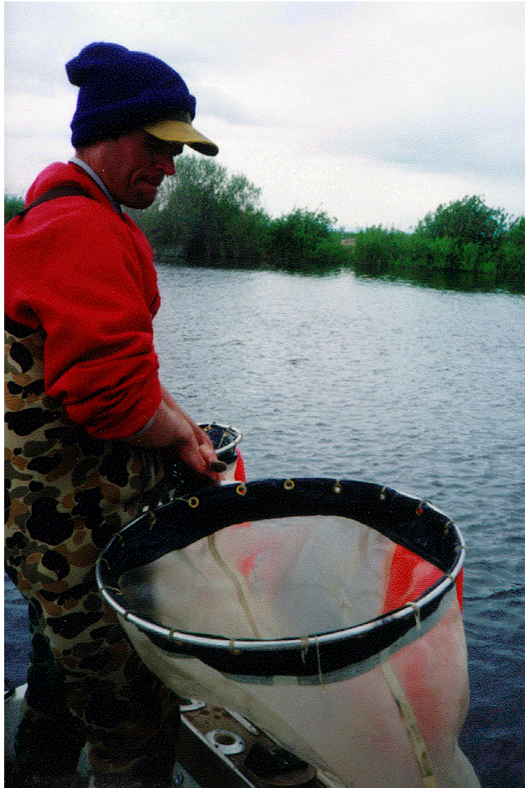
Figure B5. Twin-bongo nets used for sampling larval fishes in Upper Klamath Lake, Oregon, during June 1999 surveys. Nets being readied for deployment.
