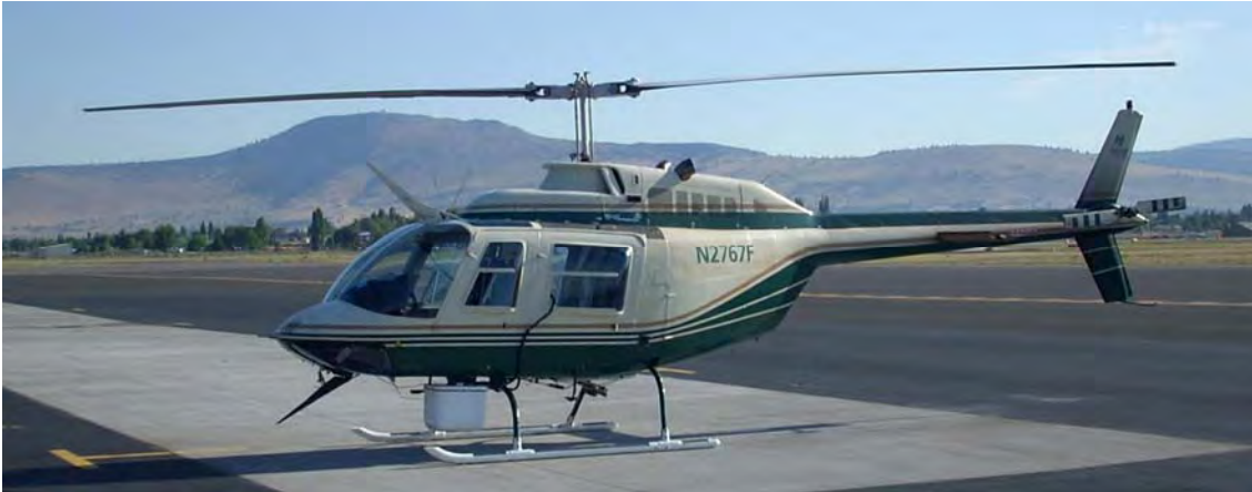
Figure 2 – Bell Jet Ranger equipped with a thermal infrared radiometer and high resolution digital camera. The sensors are contained in a composite fiber enclosure attached to the underside of the helicopter and flown longitudinally along the stream channel.
